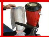
Insert a new HEPA-filter and place it carefully in the center, tighten the knurled thumb nuts but not too hard, it may damage the filter.
