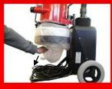
Pull out the bag so it does not get stuck in the flap.
