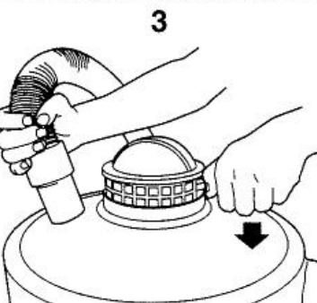
Press the filter cleaning valve hard.
